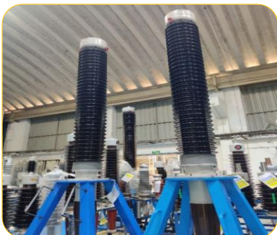
OIP Bushings with Porcelain insulators
